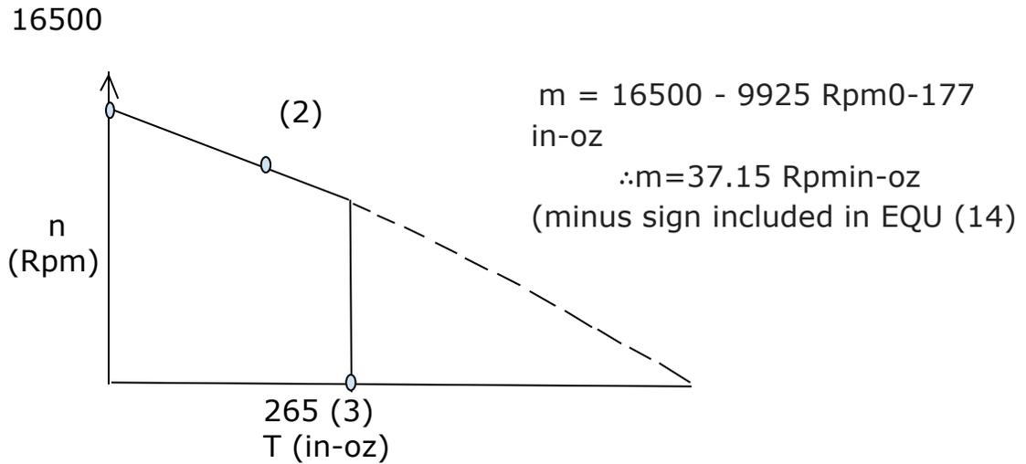
\*Line (1) - (2) is cut off at this point due to a current line limit. If the limit was not there the line would extent straight to the torque axis (depicted by the dotted line).
