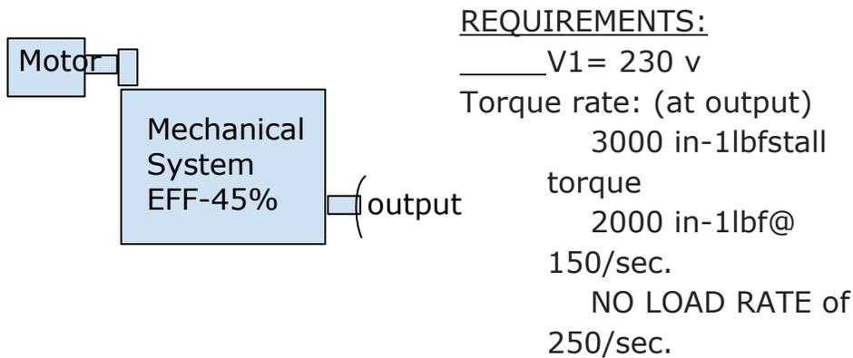
Efficiency = 45% includes the motor efficiency of 85%
