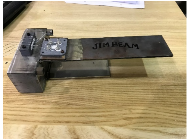
FIGURE 9. CANTILEVER BEAM JIG FOR ISOTHERMAL TESTING
