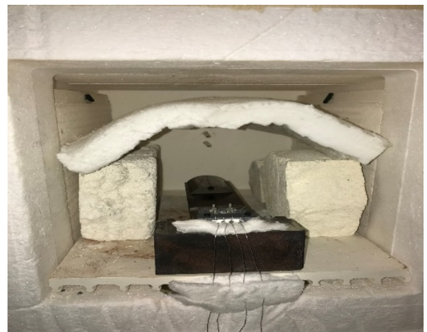
FIGURE 10. CANTILEVER BEAM JIG IN TESTING FURNACE
